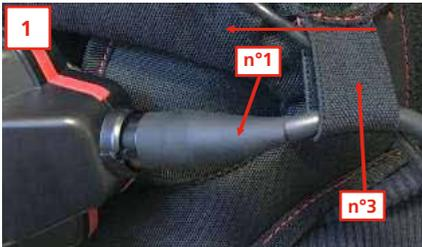
Slip the plug no. 1 through the eye hole no. 3
