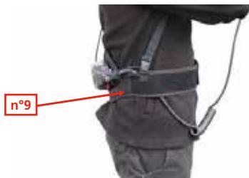
If the cable seems too long, it is possible to make it shorter. Do it by sliding the back belt vest battery door no.9, as shown above.
