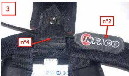
Turn the vest around and slip the fix tongue no. 2 through the central suspender ring no. 4.
